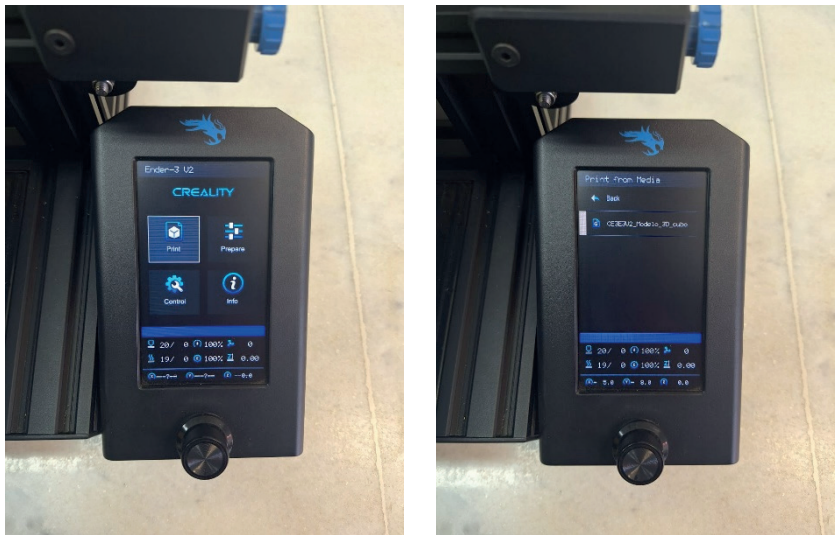
Figure 6 – Initiating the print from the control panel.
