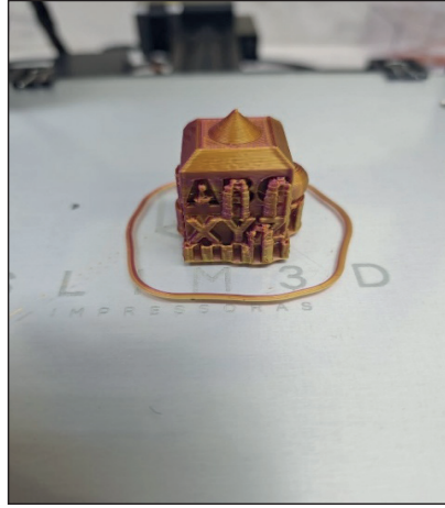
Figure 7 – Finished part before removal and support extraction.
