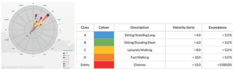
Figure 22. Weather station Data TUR_Istanbul.170600_IWEC (left), Lawson Wind Comfort Assessment Criteria (Lawson, 1978) (right).
