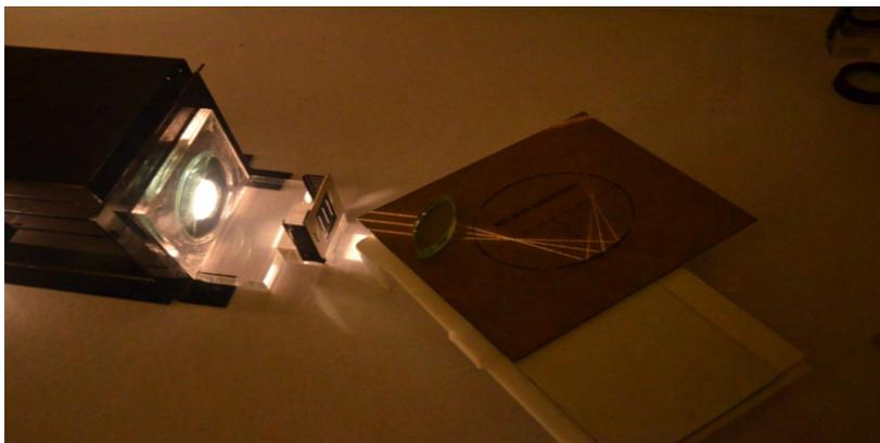
Figure 12: Component of the ellipse with the beam passing through its foci
