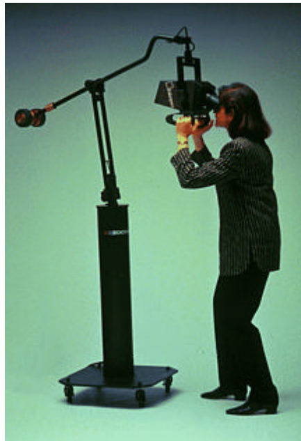
Fig. 2.07. Binocular Omni-Orientation Monitor 1 Fakespace
