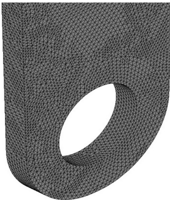
Figure 5. Mesh for the transition lower holes-legs of the fork. Source: own authorship (2020).
