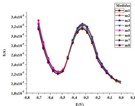
Figure 5: Repeatability test performed in water sample in the “Igarapé do Quarenta” Amazon Basin. in KCl 1 mol.L<sup>-1</sup>.  $E_{\text{dep}} = -0,2 \text{ V}$ ,  $t_{\text{dep}} = 180 \text{ s}$ ,  $t_{\text{eq}} = 60 \text{ s}$ ,  $f = 60 \text{ Hz}$ ,  $a = 70 \text{ mv}$ .
