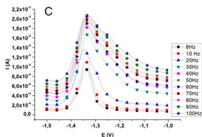
Figure 2: Relationship between frequency and the peak current obtained in standard 1 mmol.L<sup>-1</sup> metals ions solution in in KCl 1 mol.L<sup>-1</sup> for Cu<sup>2+</sup> (A), Fe<sup>2+</sup> (B) and Zn<sup>2+</sup> (C).
