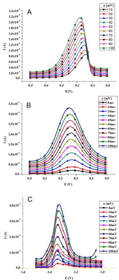
Figure 3: Dependence of the peak current with the amplitude for  $\text{Cu}^{2+}$  (A),  $\text{Fe}^{2+}$  (B) and  $\text{Zn}^{2+}$  (C)  $1 \text{ mmol.L}^{-1}$  in  $\text{KCl } 1 \text{ mol.L}^{-1}$  solutions.
