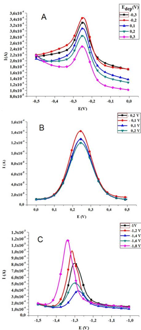
Figure 1: Relationship between deposition potential and peak current obtained in standard  $1 \text{ mmol.L}^{-1}$  metals ions solution in KCl  $1 \text{ mol.L}^{-1}$  for  $\text{Cu}^{2+}$  (A),  $\text{Fe}^{2+}$  (B) and  $\text{Zn}^{2+}$  (C).
