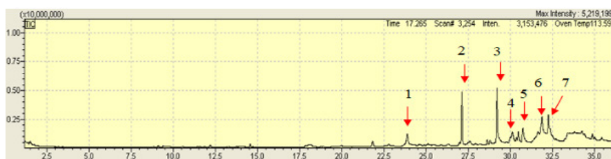
Figure 1: Chromatogram containing the peaks of the substances isolated through the immersion method.
