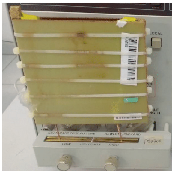
Figure 3. Sample holder with resin installed in HP 16047C Test Fixture
