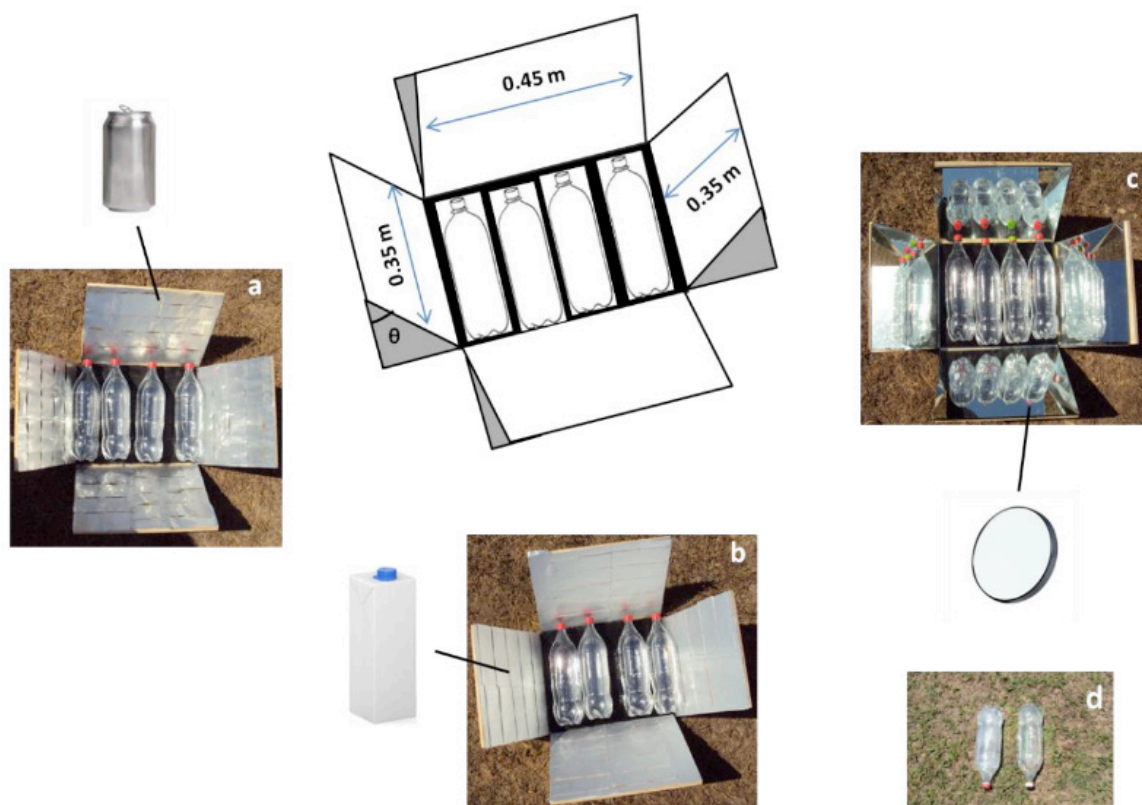
Figure 1. Solar energy concentrators (SOCOs) to improve heat transfer during water solar disinfection. a). SOCO-aluminum foil from beverage cans, b). SOCO-aluminized tetra pak packages, c). SOCO-mirror, and d). SODIS.
