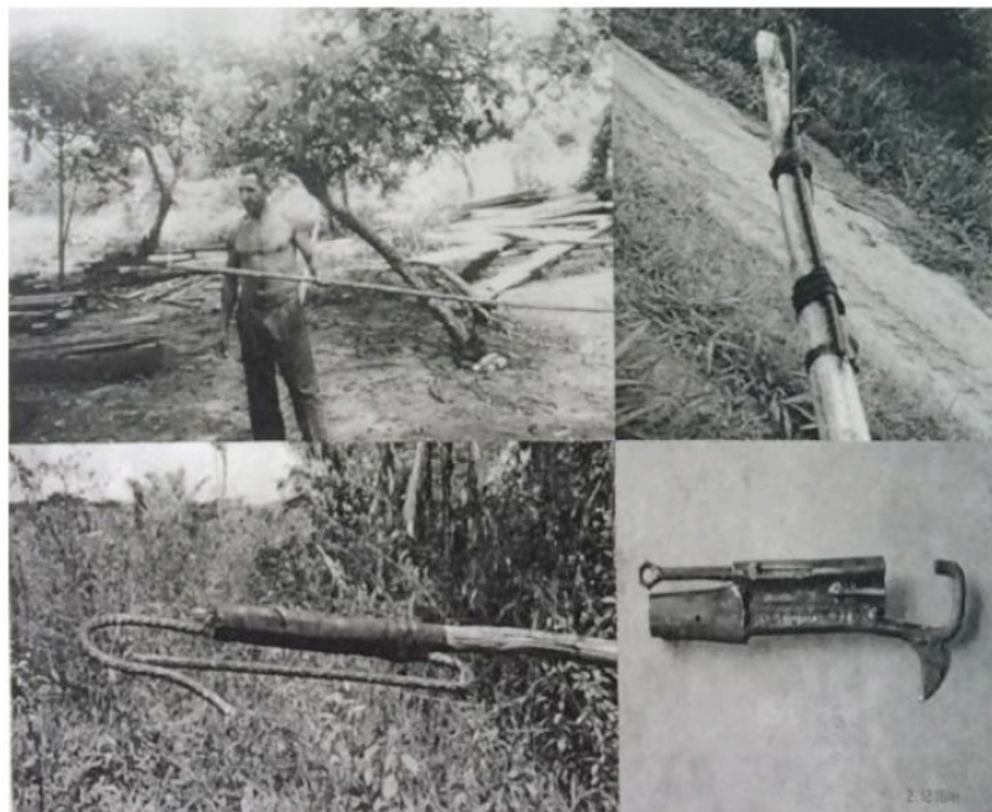
Figure 2. Açai bunch collector made of wood with its variations in the cutting system.
