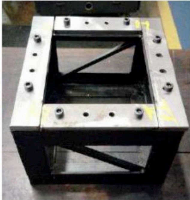
Figure 1. Support for fixing the pure aluminum sheet.
