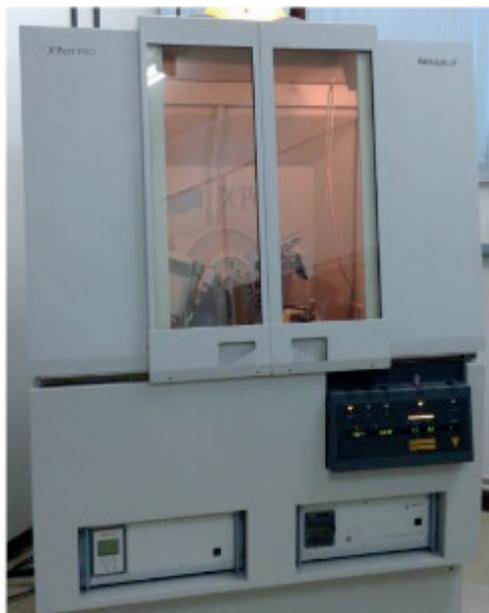
Figura 3. Difratorômetro PANalytical X'PERT PRO MPD (PW 3040/60)
