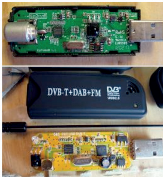
Figure 2. SDR hardware adapter. (Superkuh, 2017)
