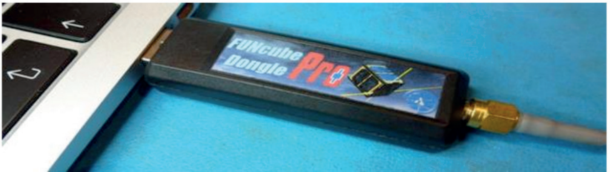
Figure 3. Funcube Dongle Pro Plus connected to computer.
