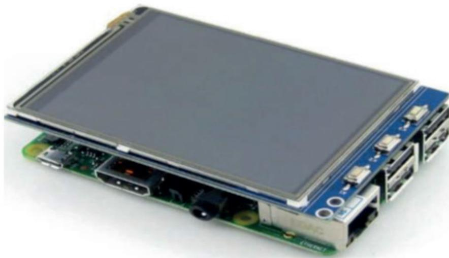
Figura 3. Display LCD touchscreen TFT de 3.2”
