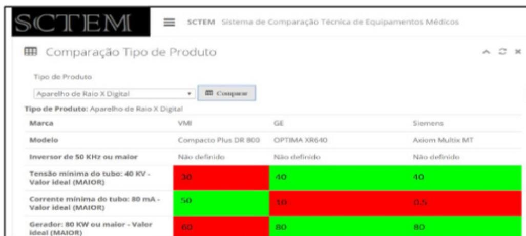
The screenshot shows the SCTEM interface with a dropdown menu set to 'Aparelho de Raio X Digital' and a 'Comparar' button. Below, a table compares three models: VMI Compacto Plus DR 800, GE OPTIMA XR640, and Siemens Axiom Multix MT. The table includes technical specifications and their values for each model, with red highlighting indicating values below the ideal and green highlighting indicating values above the ideal.
