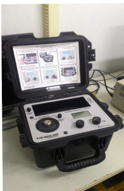
Figura 5. 9100D Portable Shaker Vibration Calibrator .
