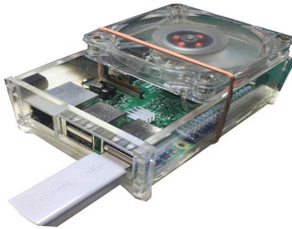
FIGURA 4: Raspberry Pi 3 com cooler.
