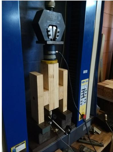
Figure 1: Test for determination of Slip Module ( $K_{ser}$ )
