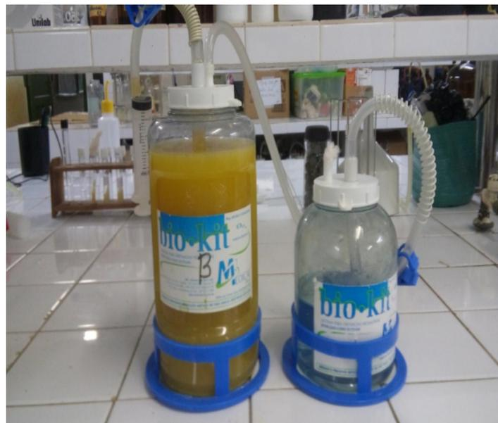
Figure 1 – Bioreactor containing common orange must.
