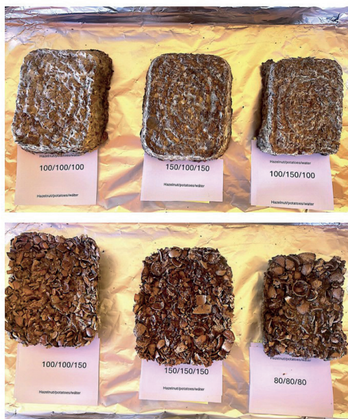
Figure 4: Insulation panels made of biomaterials. Showing the top and the side of them.
