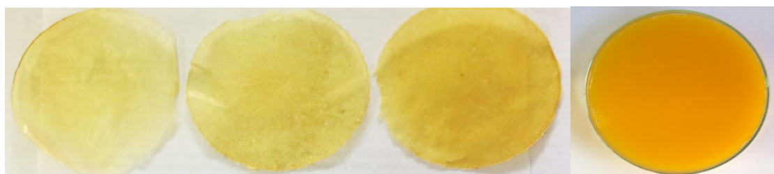
Figure 7: NCCH/B films with 1:0,5, 1:1 and 1:2 of Buriti oil and polymer content, and NCCH/B gel-like solution, respectively. Source: FIGUEIREDO et al, 2018. The synthesis of NCCH/B biocomposite is not characterized as an ordinary mixture of biopolymer and oil, but a new method of obtaining the material studied. Since this composite has been obtained in an aqueous medium and the difference of polarity, composition of the substances, different densities and structures support the idea of complexation. Buriti oil presents in its composition many fatty acids containing ions compatible with the amine group from chitosan, which justifies the complexation with one or more of these fatty acids, still not identified.
