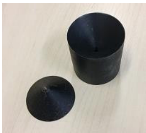
Figure 4 – Anticlepsydra and one of the cones that form the clepsydra made of carbon steel
