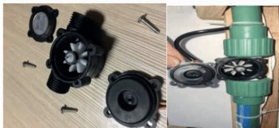
Figure 15. Exploded view of the YF-S201 flux sensor for the experimental physical model.
