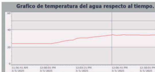
Figure 20. Graph in the HMI shows the heating time from 24 to 34 0C with the tank at 28.8% without discharge. Source: Own elaboration.
