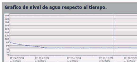
Figure 18. HMI graph of level control from 83.3% to 28.8% with discharge. Source: Own elaboration.
