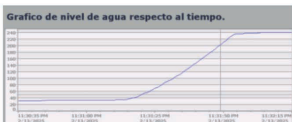
Figure 16. HMI graph of tank filling time from 12.5% to 83.3% with closed tap. Source: Own elaboration.
