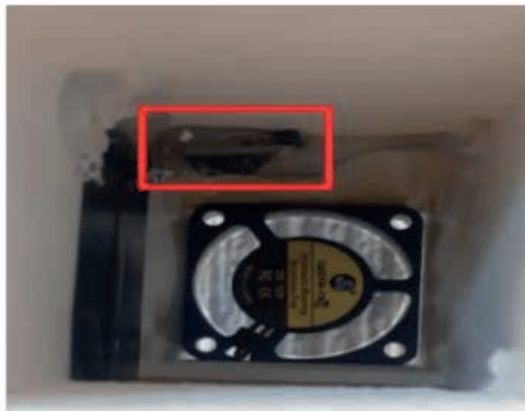
Figure 8. Location of the level sensor inside the air circulation duct. Source: Own elaboration: Own elaboration.
