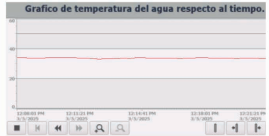
Figure 21. HMI graph showing temperature control at 34 0C with tank at 93.7% with discharge. Source: Own elaboration.
