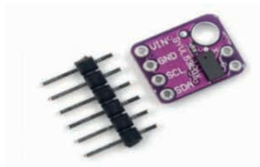
Figure 6. Diagram of the VL53L0X level sensor. Source: Own elaboration.
