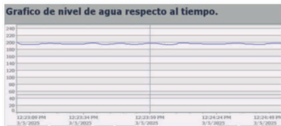
Figure 17. Graph in the HMI on the level control at 83.3% with discharge. Source: Own elaboration.
