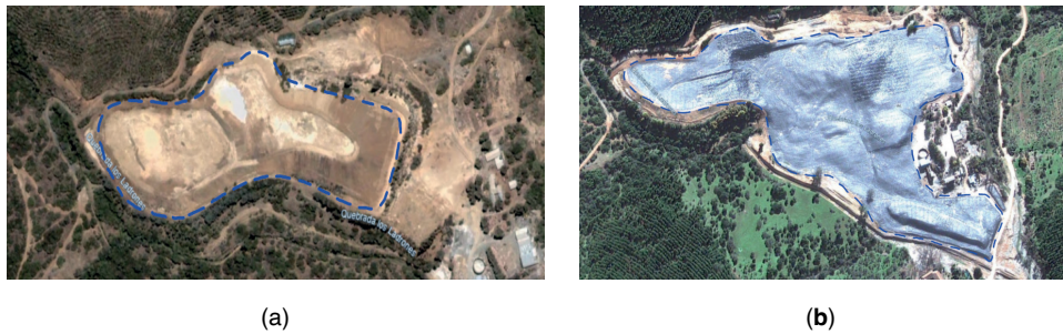
Figure 5. Geometry of the Las Palmas tailings dam: (a) Geometry of the dam before the failure (2005); (b) Geometry of the dam after the failure (2010).
