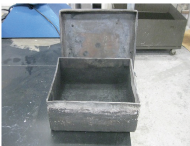
Figure 2. Shows the metal box where AISI 1018 steel samples were placed, and the charcoal and barium carbonate mixture, once filled, was covered, sealed with clay and placed in the furnace for treatment.
