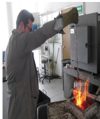
Figure 4. Extraction of the steel samples from the box to be subsequently quenched and tempered in mineral oil.
