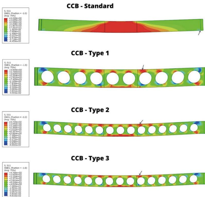
Figure 11. Longitudinal stress (S11) distribution (MPa).
