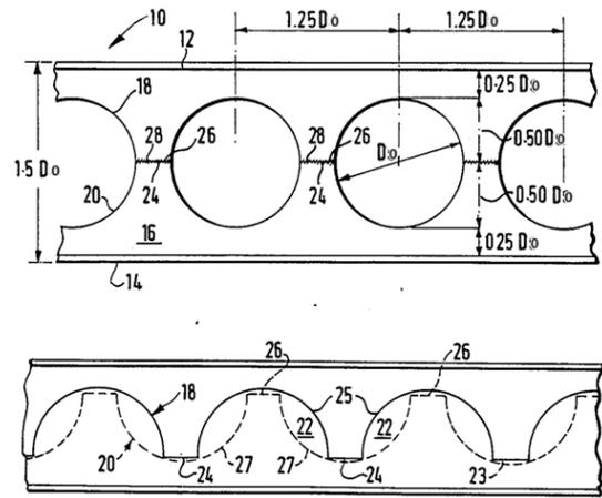
Figure 2. Circular cellular beam featured in British patent n° 4894898 (Walker, 1990).
