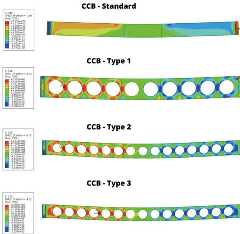
Figure 12. Shear stress (S12) distribution (MPa).
