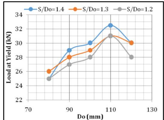
Figure 5. Variation in yield load for different  $S/D_0$  and  $D/D_0$  ratios for cellular beam (Jamadar & Kumbhar, 2015).
