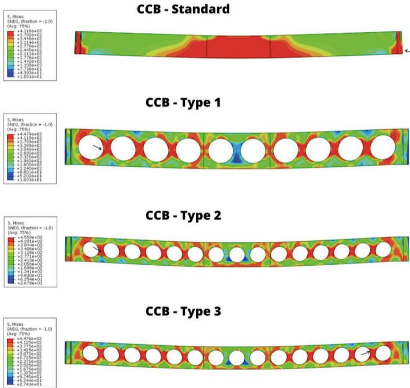
Figure 10. Von Mises stress distribution (MPa).
