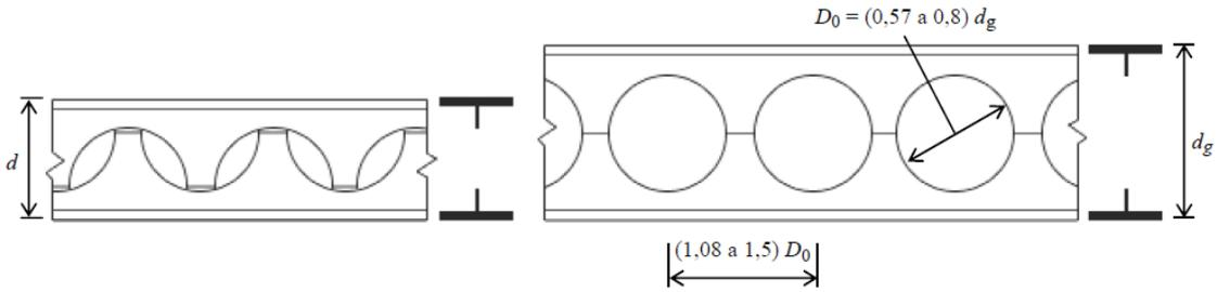
Figure 3. Geometric properties of cellular beams (Harper, 1994).
