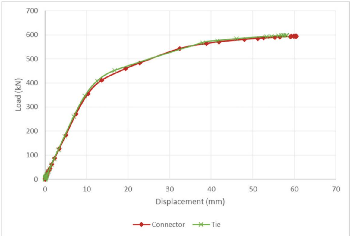
Figure 9. Load vs. Displacement curve on CCB standard.
