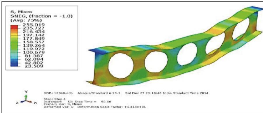
Figure 4. Variation in stresses of the optimized cellular beam (Jamadar & Kumbhar, 2015).
