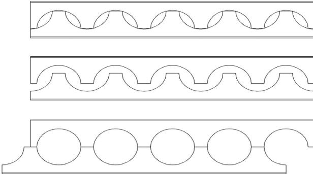
Figure 1. Manufacturing of castellated beams.
