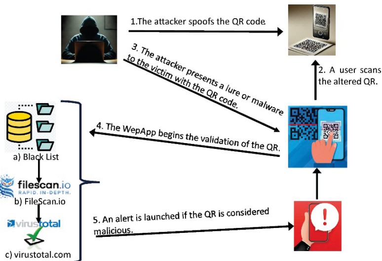
Fig 5. Detection method for compromised QR codes based on a blackList.
