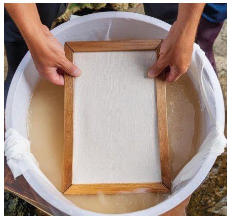
Figure 4 - Shaping the handmade sheet of paper Source: Authors' personal archive.
