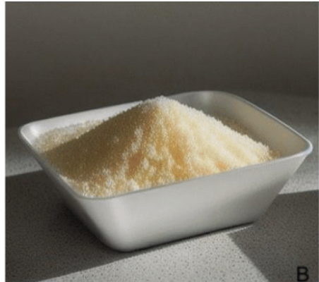
Figures 3- Preparation of paper pulp and incorporation of cellulose fiber Where: A - Homogenization of recycled paper; B - Cellulose fibers flocked in a solid state. Source: Authors' personal archive
