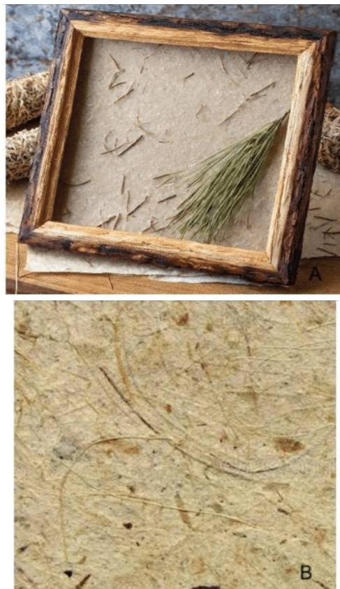
Figures 7A and 7B - Images of the sheets of paper with acicles not adhered to the pulp.
