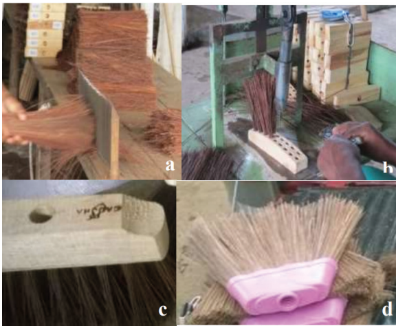
Figure 8. a) Selection and cleaning; b) stapling of clean vegetable fiber; c) “stump” brooms; and d) brooms sheet (Pimentel 2020).
