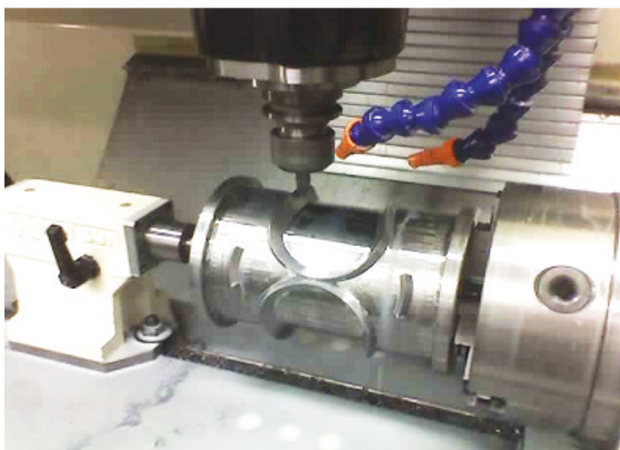
Figure 2 - Milling process using MQF technique
