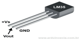
Figure 11: LM35 temperature sensor
