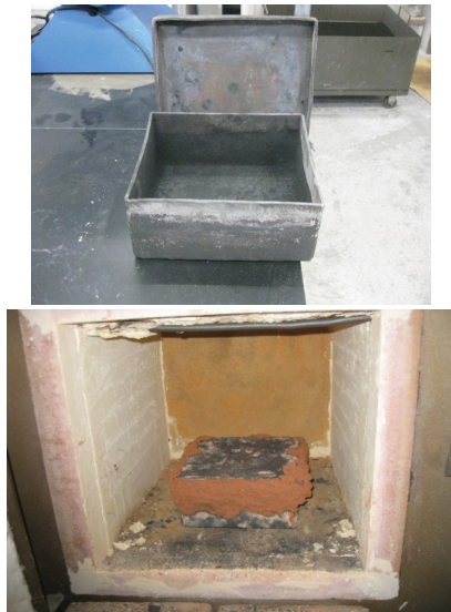
Figure 2. Shows the box for treatment and when it is already lined with clay ready for thermochemical treatment.
