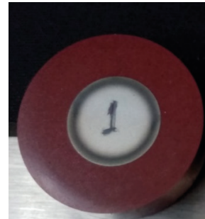
Figure 5. Shows the specimen that was mounted for mapping to determine the depth of cementation.
