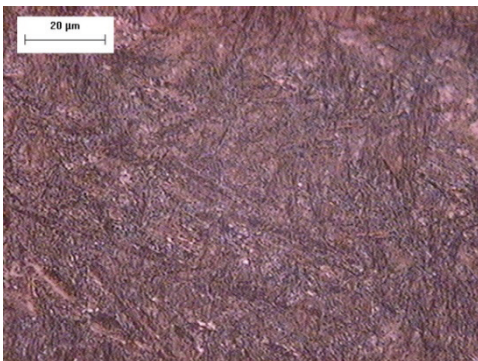
Photomicrograph 1.- Piece 1, Surface , the microstructure consists of a matrix of tempered martensite, 500x, chemical attack: Nital 5%.
