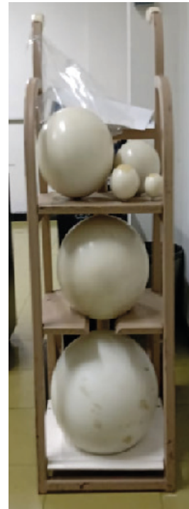
Figure 2: NL/NLMIR Bonner spheres.
