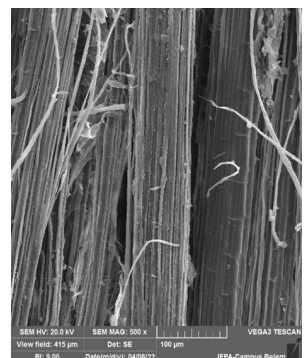
Figure 7 - Fractography of timbó-açu fiber. In natura. 500x
