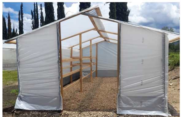
Figure 1. Zenith type solar dryer for coffee drying, used in the study.
