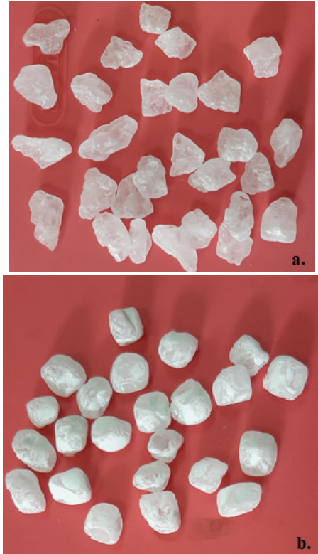
Figure 2. a) Irregular particles size T8 and b) Rounded particles size T8.
