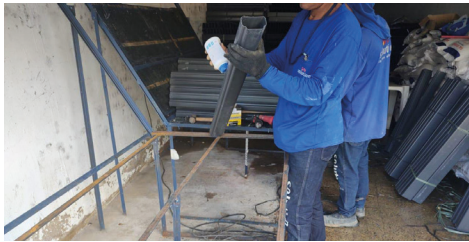
Figure 7: Application of sticky adhesive
