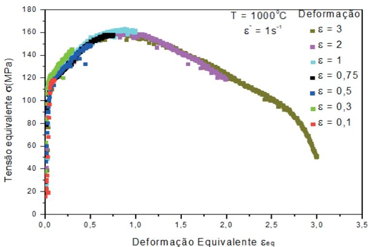
Figure 7. Curves and microstructures for tests conducted at 1000 °C with a deformation rate of 1 s<sup>-1</sup> using cold rolled steel
