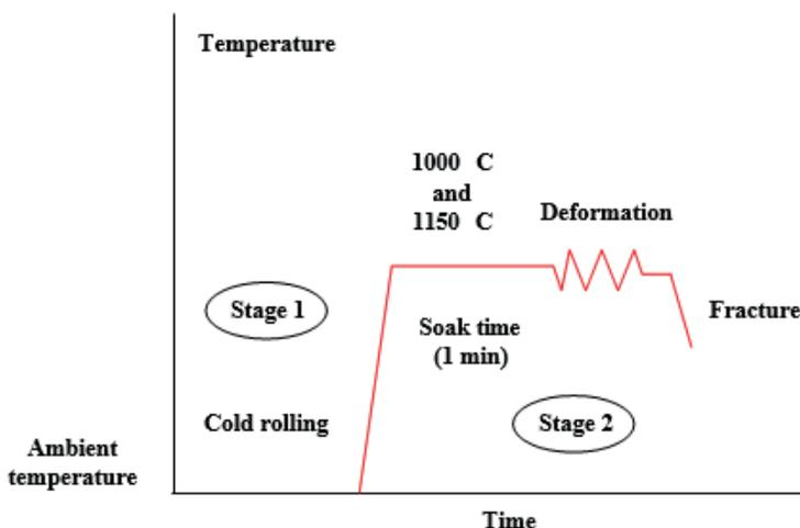
Figure 3. Schematic representation of cold rolled steel tests.
