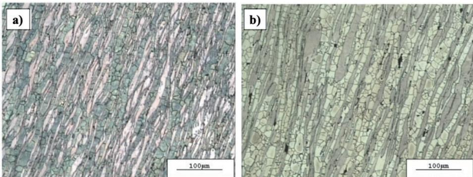
Figure 6. Microstructures for tests performed at 1150 °C with deformation rates of (a) 0.5 s<sup>-1</sup> and (b) 1 s<sup>-1</sup> using cold rolled steel deformed  $\epsilon_f = 3.0$  and  $\epsilon_f = 2.5$ , respectively
