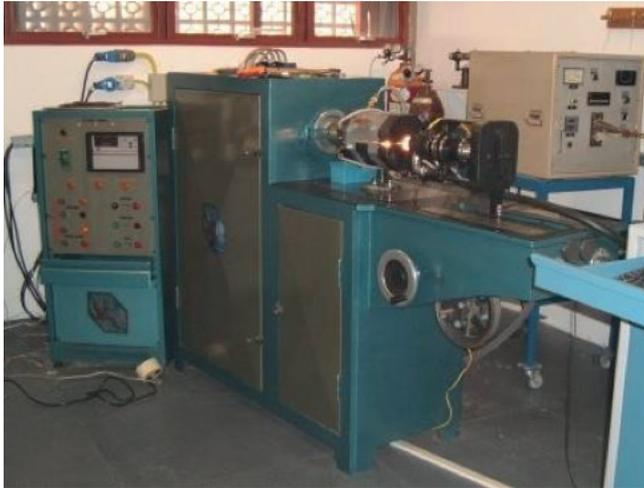
Figure 2. Hot torsion test machine
