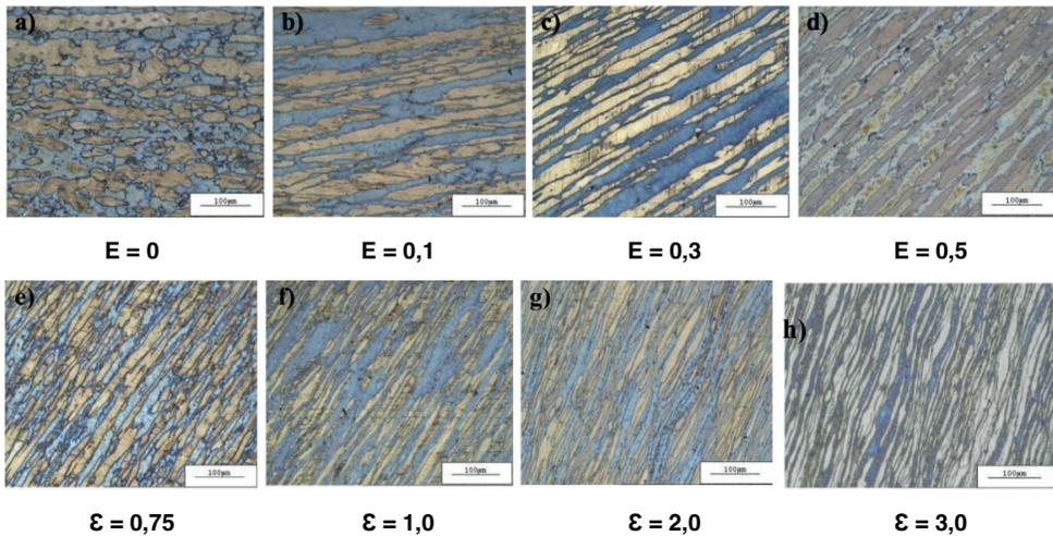
Figure 8 - Cold rolled duplex stainless steel microstructures with different deformations; test temperature 1000 °C and deformation rate 1 s<sup>-1</sup>
