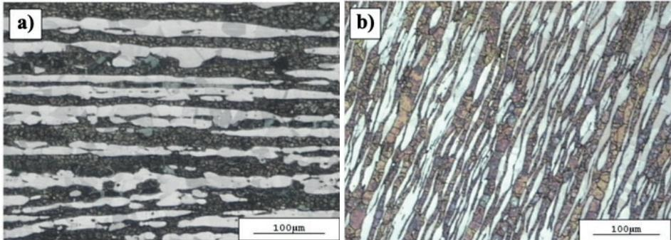
Figure 4. Relative microstructures for the test carried out at 1150 °C with a deformation rate of 0.3 s<sup>-1</sup> and deformed until fracture using cold rolled steel, where (a) represents the initial microstructure before deformation and (b) represents the final microstructure deformed fracture  $\epsilon_f=2.2$
