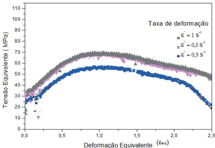
Figure 6. Plastic flow curves from tests performed at 1150 °C with deformation rates of 0.3 s<sup>-1</sup>, 0.5 s<sup>-1</sup> and 1 s<sup>-1</sup> using cold rolled steel.
