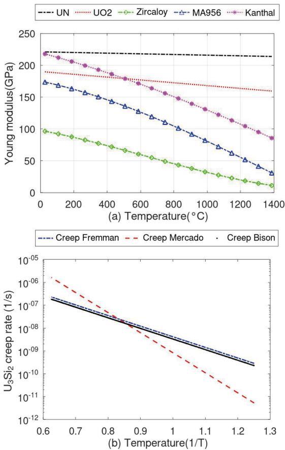
Figure 2. (a) Young modulus of ATF materials, (b) creep rate of U<sub>3</sub>Si<sub>2</sub>
