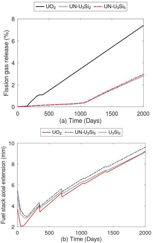
Figure 4. (a) fission gas release and (b) fuel axial extension
