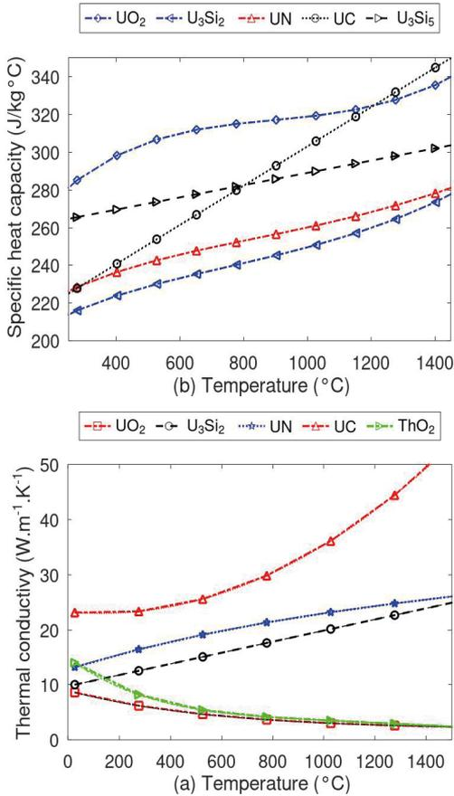
Figure 1. (a) Thermal conductivity of ATF fuel and (b) specific heat capacity.
