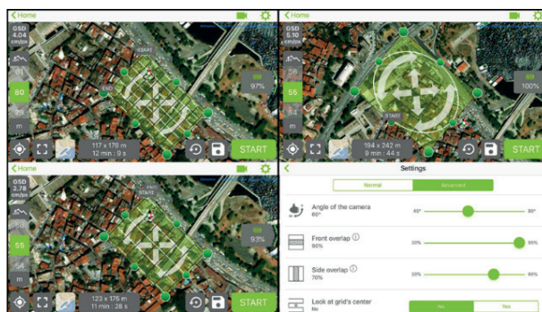
Figure 9. Flight 2 plan and settings (Pix4D App), oblique flights (left), Circular path flight (upper right), oblique flight settings (lower right).
