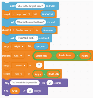
Figure 11 : Algorithm for calculating the area of a trapezoid.
