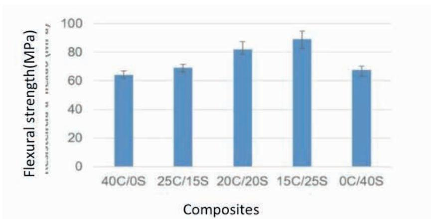
Figure 5 – Flexural strength of the five different composites. Adapted from (ATMAKURI et al., 2021)
