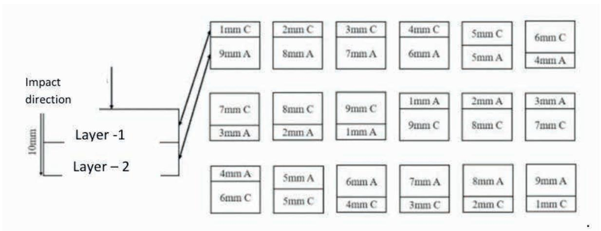
Figure 3 – Aramid/carbon hybrid composite stacking sequences. Adapted from (XU et al., 2023)
