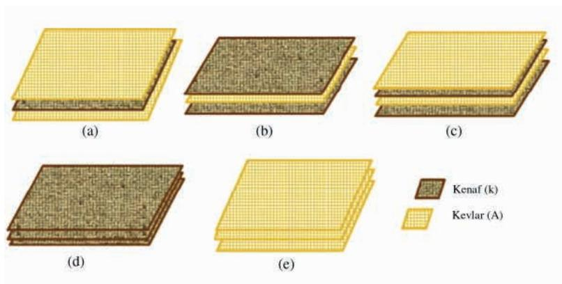
Figure 6 – Illustration of the configuration of the composites (a) A/k/A (b) k/A/k (c) A/k/A/k (d) k/E and (e) Kevlar/epoxy. (YAHAYA et al., 2015)
