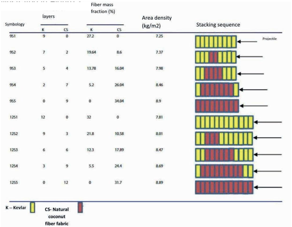
Figure 7 – Symbol of laminates and their corresponding weight fraction and stacking sequence. Adapted from (NAVEEN et al., 2019)
