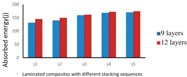
Figure 8 - Energy absorption of laminated composites. Adapted from (NAVEEN et al., 2019)
