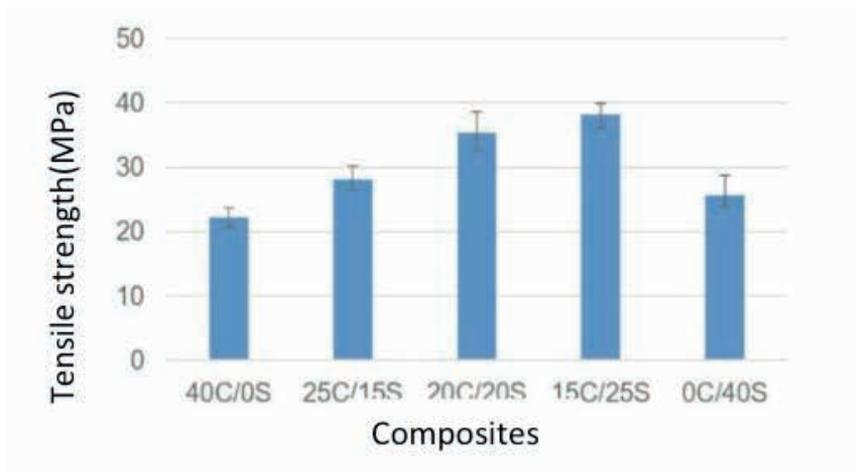
Figure 4 – Tensile strength of the five different composites. Adapted from (ATMAKURI et al., 2021)
