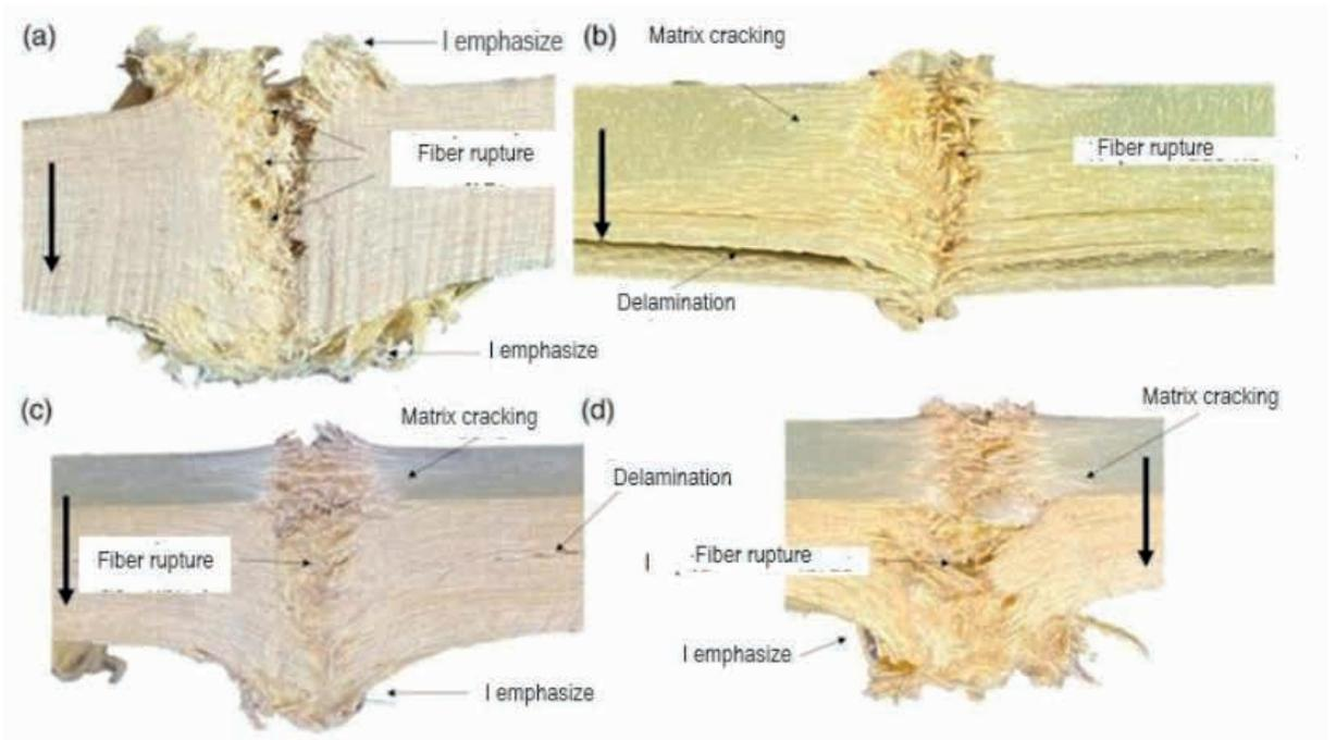
Figure 2 – Deformation mechanisms of composites (a) A, (b) E, (c) H1, (d) H2. Adapted from (ÜSTÜN; TOKSOY; TANOĞLU, 2022)
