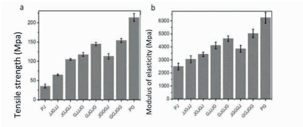
Figure 10 – Tensile strength (a) and Modulus of elasticity (b) of hybrid composites reinforced with jute and glass fiber. Adapted from (GHANI et al., 2022)
