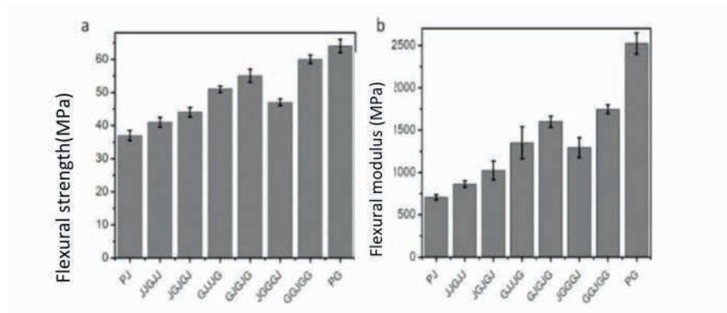
Figure 11 – Flexural strength (a) and flexural modulus (b) of hybrid composites reinforced with jute and glass fiber. Adapted from (GHANI et al., 2022)
