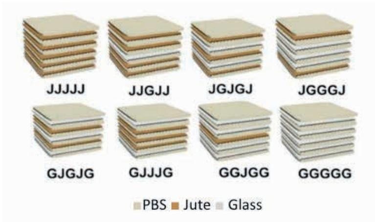
Figure 9 - Jute/glass fiber stacking sequence. Adapted from (GHANI et al., 2022)
