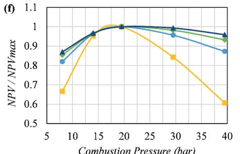
Figure 7 - Influence of Annual Interest Rate, Annual Operating Hours and Electricity Price over  $NPV \div NPV_{max}$  dependence upon GT combustion pressure ( $P_{comb}$ ) for LGTW-CONV (a-c) and LGTW-BECCS (d-f)
