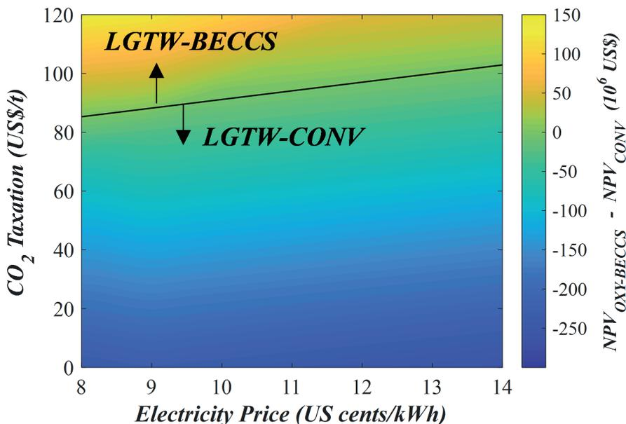
Figure 10 - Delta NPV ( $NPV_{OXY-BECCS} - NPV_{CONV}$ ) as a function of electricity price (¢/kWh) and CO<sub>2</sub> tax level (USD/t).  $NPV_{CONV} \equiv NPV$  of LGTW-CONV base process.  $NPV_{OXY-BECCS} \equiv NPV$  of LGTW-BECCS base process
