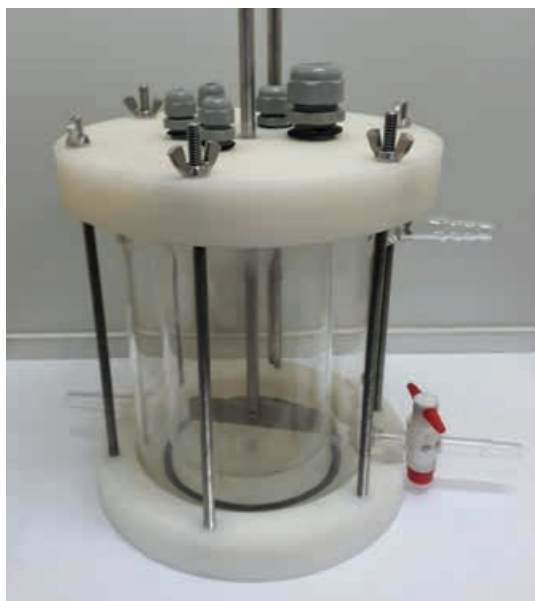
Figure 5 - Complete jacketed bioreactor developed.
