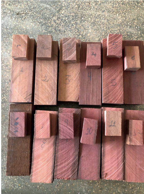
Figure 3 - Test specimens for moisture content testing and the respective specimens to be broken.
