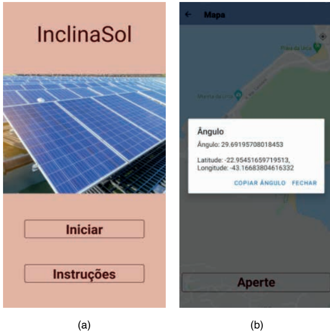
Figure 2 - (a) displays the initial screen of the InclinaSol app, while (b) shows the indication of the optimal angle for solar panel installation based on the provided geographical coordinates.
