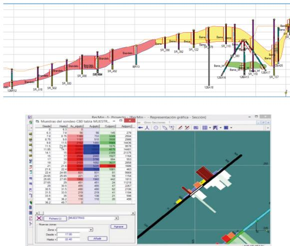
Figure 3. Representation of geological profile from drilling data (RECMIN©).
