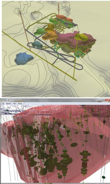
Figure 4. 3D visualization of subsoil mining works and drillings with lithological information (RECMIN©).
