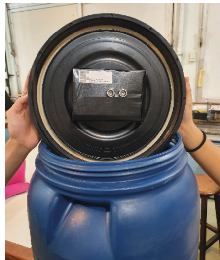
Figure 4: Small-scale reservoir for simulating the monitoring of water consumption and supply flows.
