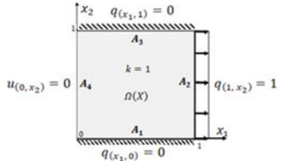
Figure 1 - Temperature gradient on the square plate
