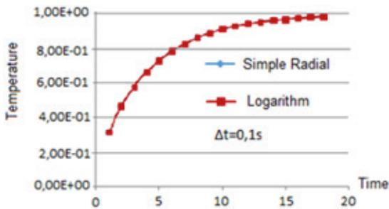
Figure 3 - Comparison of MECID response curves over time for temperature on the right edge
