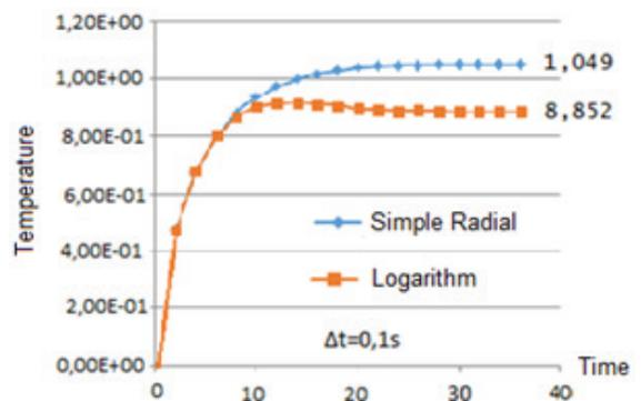
Figure 2 - Comparison of MECDR response curves over time for temperature on the right edge
