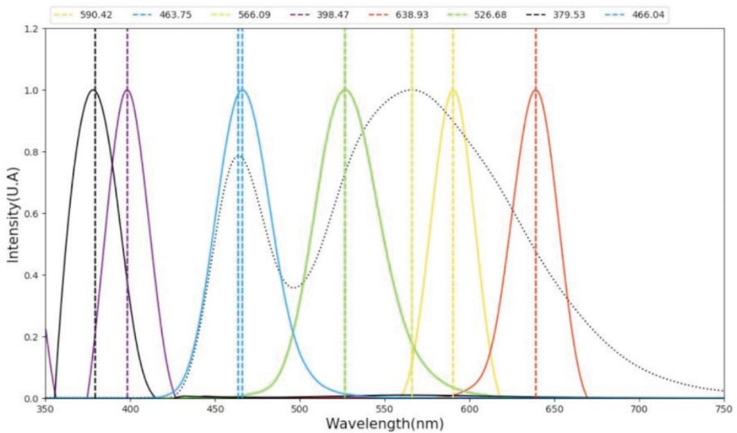
**Figure 1.** LED emission spectra at different wavelengths.
