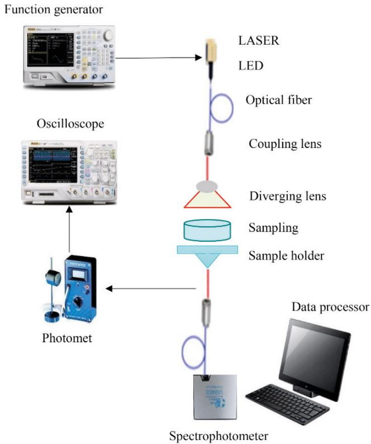
**Scheme 1.** Experimental setup for optical characterization in biological tissues
