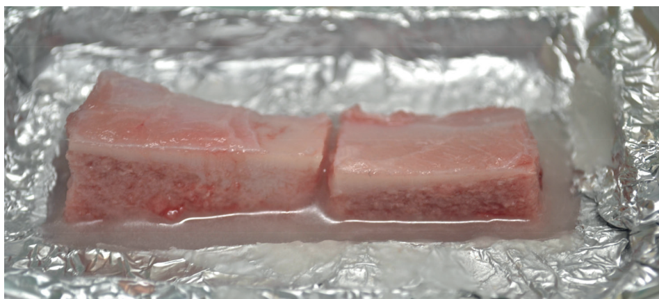
Figure 5 – Swine iliac bone specimens positioned on resin during the polymerization process.
