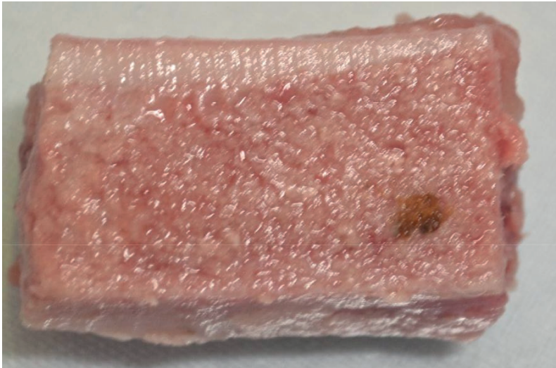
Figure 3 – Selection of parts with bone cortical thickness ranging between 1.7 and 2 mm and elimination of specimens with thicknesses outside this range.
