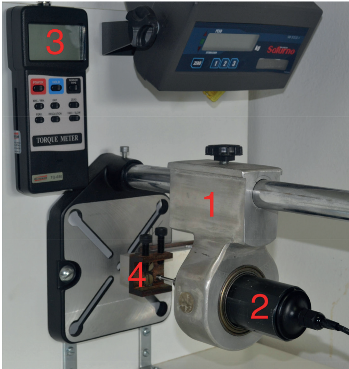
Figure 7 – Device used for inserting the miniscrews in swine iliac and bovine tibia specimens. 1 - Insertion reference; 2 - Digital axial torque wrench (torque sensor) with attached miniscrew wrench; 3 - Torque sensor display; 4 - Vise for seizure and stabilizing specimens for inserting miniscrews.
