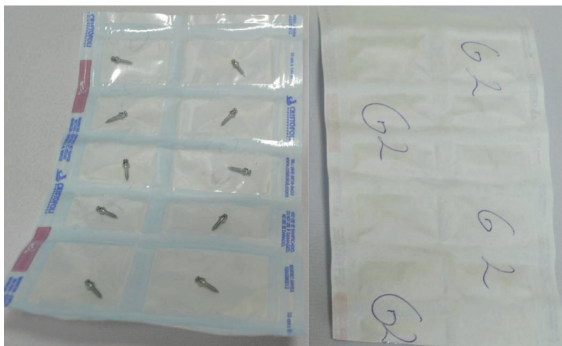
Figure 10 – Miniscrews wrapped individually and identified by group, ready for sterilization.
